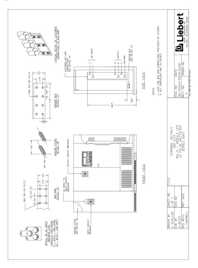
Figure 31 Terminal Details, 625 & 750 kVA Modules, 6-Pulse and 12-Pulse
